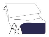
3.Power on the printer, make sure the white tracing paper is face down and the blue transfer paper is face up, insert the paper from the back of printer, then the printer will feed the paper automatically.
