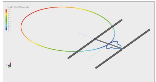
Antenna 2: Typical horizontal characteristic for the directional dipole antenna, computed for the far field.
