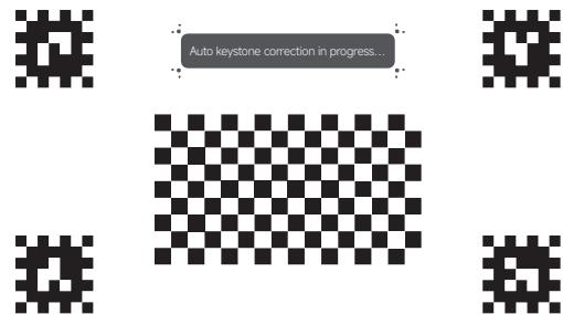
**Note:** After auto keystone correction is completed, you can also press the confirm button on the remote control to enter manual keystone correction, and use the remote control to fine-tune the image corners for correction.
