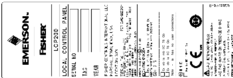
Figure 9. LCP200 ATEX/IECEx Nameplate, Explosion-proof, Group IIC
