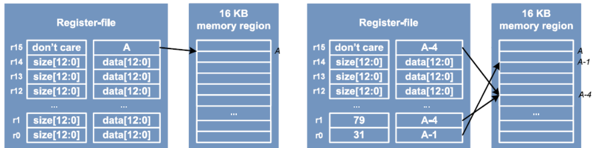
Figure 12-18. Left: Register File State before ALLOC_MEM Instructions; Right: Register File after ALLOC_MEM Instructions
