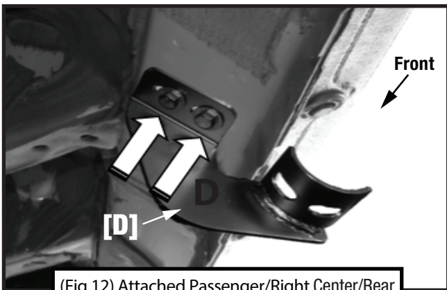
(Fig 12) Attached Passenger/Right Center/Rear Bracket [D] at rear mounting location
