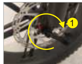
5. Rotate and disassemble quickly, lock the front fork
