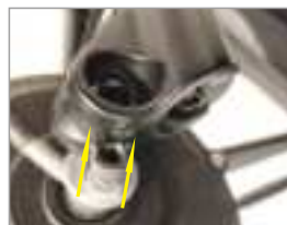
3. Install the front fork and insert the adjusted front wheel axis into the front fork slot
