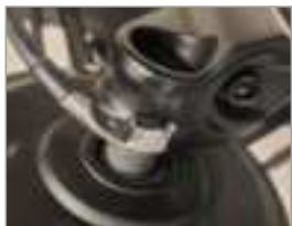
4. As shown in the figure, install the front fork
