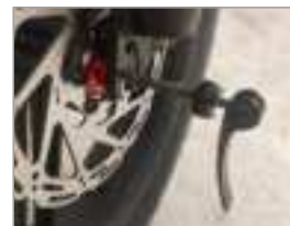
3. Insert the quick release axle into the front wheel as shown in the figure
