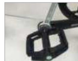
5. Take out the pedal with the letters "R" and "L", align it with the crank hole and lock it with a wrench
