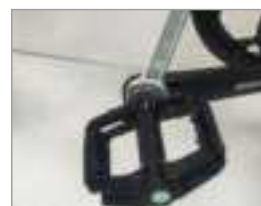
3 Take out the pedal with the letters "R" and "L", align it with the crank hole and lock it with a wrench
