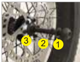
2. Install bearings as shown in the diagram
