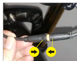
4. Connect the light cable (note that the direction of the arrow needs to correspond)
