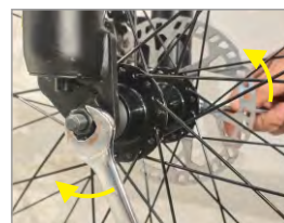
6. Tighten both ends of the axis as indicated by the arrow in the figure
