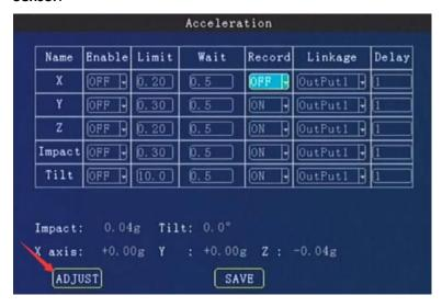
Click on **ADJUST** to zero the calibration and **SAVE** to confirm the settings.
