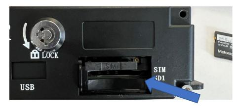
Remove the SIM card holder, to do this push the small button at the top right of the SIM card slot.
