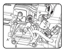
A- Spark plug B- Spark plug cap
