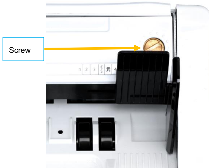
Figure 2-6 The Adjustable Screw
