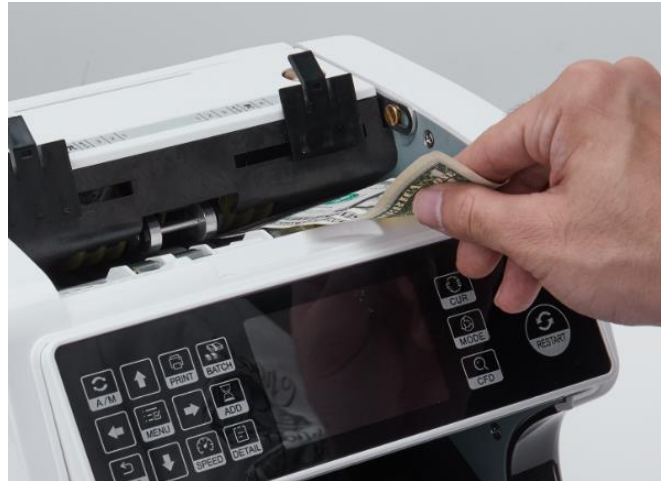
Figure 2-11 Using a banknote to check the gap between the rollers
