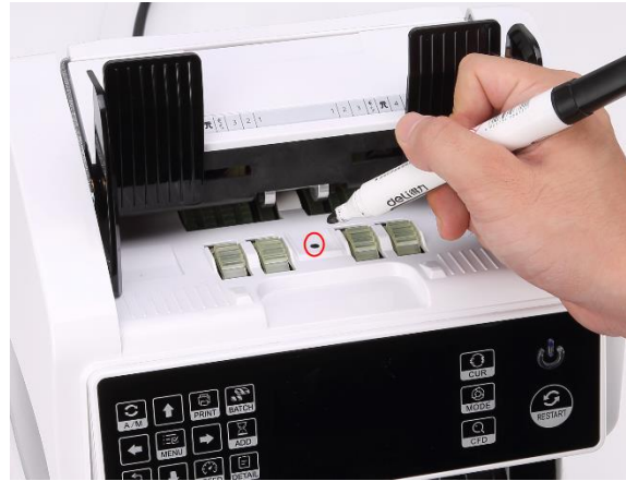
Figure 2-5 Using marker pen to decrease the sensitivity of the hopper sensor
