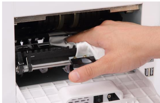
Figure 2-21 Clean the Lower CIS
