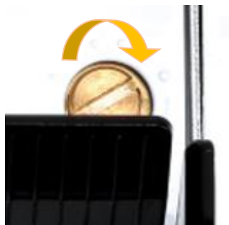
Figure 2-7 Rotate the Screw to Increase the Feeding Gap
