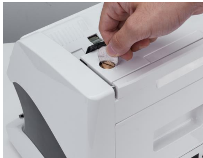
Figure 2-12 Using a coin to adjust the gap
