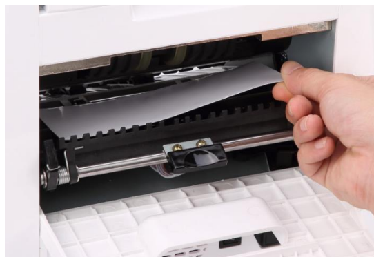
Figure 2-23 Place the CIS Calibration Paper
