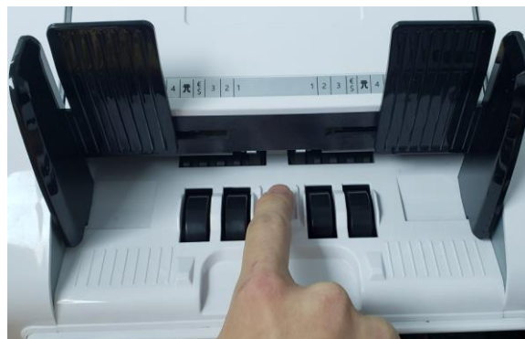
Figure 2-16 Touch the Hopper Sensor
