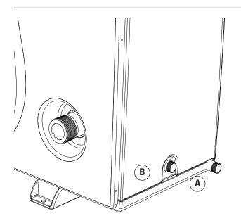
A: CONDENSATION WATER DRAIN PIPE
