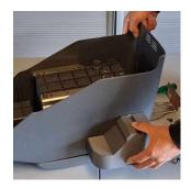
5. Insert the metal support bracket, line up and start threading the 2 x Phillips head screws through the metal support bracket and into the new cupholder.
