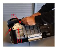
3. Remove the Phillips head screw on the outside of the console and remove the metal support bracket and factory cupholder.
