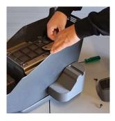
6. Position the metal support bracket into place and insert and tighten the 1x Phillips head screw to attach the metal bracket to the console.
