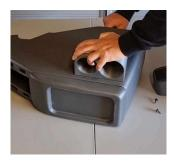
8. Insert and tighten the exterior Phillips head screw under the cupholder, through the console and onto the metal support bracket through the factory hole. Be careful not to over tighten this screw as it will tighten the bottom to the console but create a gap at the top of the console.
