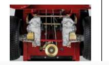
CONTROLS Twin independent ZT2800 hydrostatic drives with integrated charge pumps allow precise, multi-directional cutting control while hydraulic dampers eliminate "jerky" operation and arm fatigue typical of spring-return designs.
