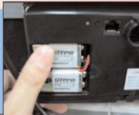
Figure 6: Install the 9 volt batteries
