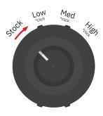
**Low:** — Towing heavy and low traction situations.
