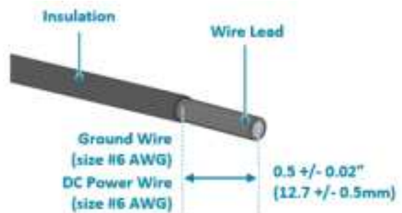
6-AWG green-and-yellow wire for grounding 6-AWG DC power wire
