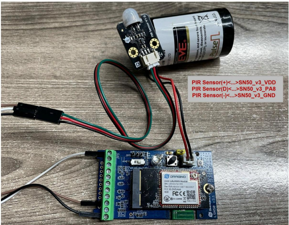
**Note: LoRaWAN wireless transmission will infect the PIR sensor. Which cause the counting value increase +1 for every uplink. User can change PIR sensor or put sensor away of the SN50\_v3 to avoid this happen.**
