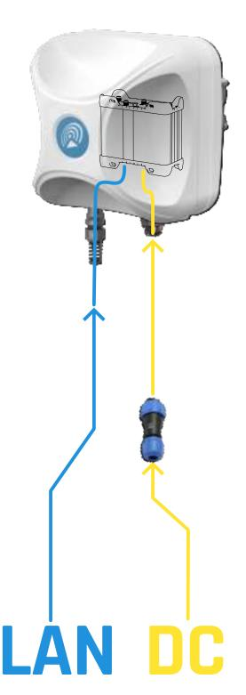
Please note that for Teltonika RUTX series, the DC power source ranges from 9 to 50 VDC, while for the RUT series it is 9 to 30 VDC.
