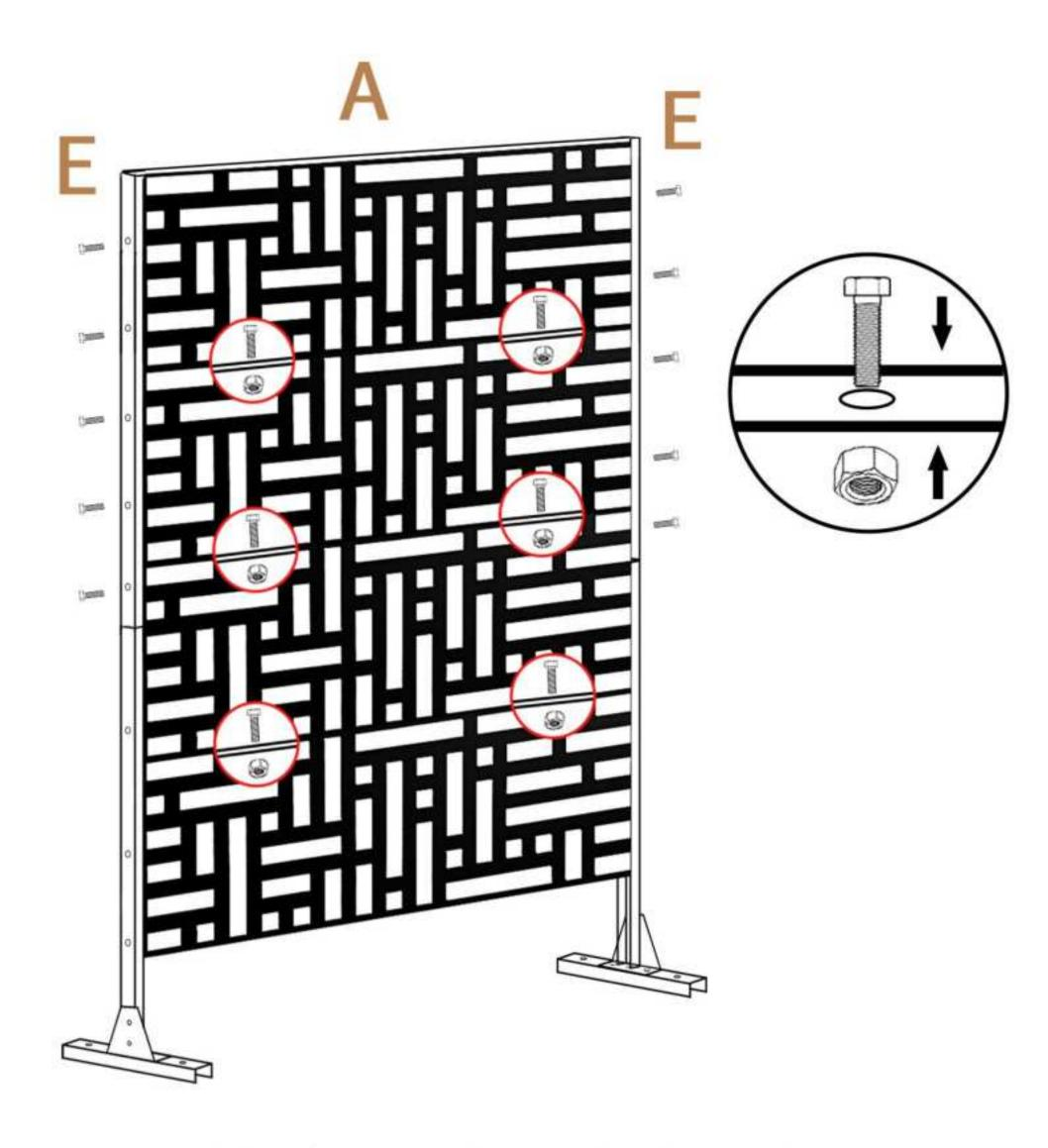
Fix the remaining 2 pieces A in E with screws and nuts
