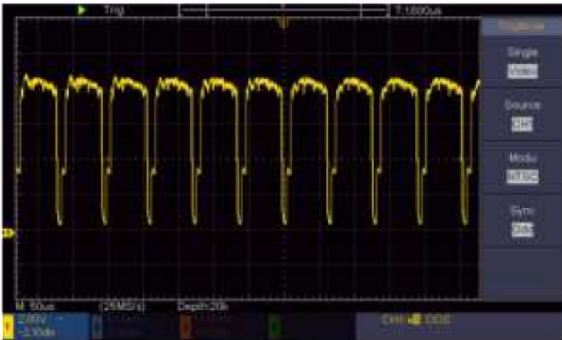
Figure 6-7 Waveform Captured from Video Field Trigger
