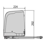
Electromechanical operator with articulated arm for residential use, for swing gate leaves of up to 2 metres and 200 kg. Ideal for any installation requirements, makes it easy to solve problems linked to large pillars thanks to the lever system. Operator-integrated control unit, limit switch and mechanical stops.
