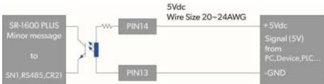
Figure 9-4. Application diagram of dry contact pin14~13(Minor)
