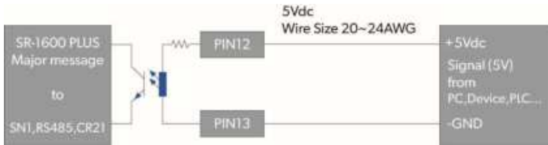
Figure 9-3. Application diagram of dry contact pin12~13(Major)
