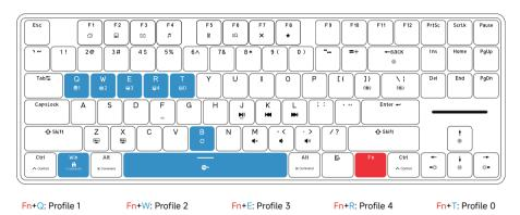
Fn+B: Press long until light of the keyboard blinks, the keyboard reset to the factory default settings.
