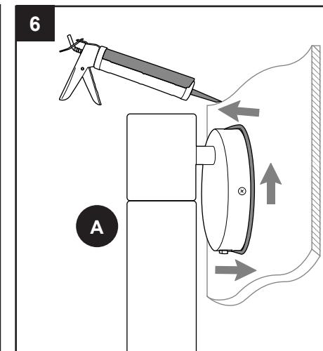
Caulk mounting surface of A with silicone weather sealant (not included).
