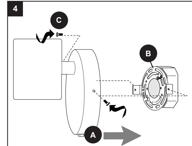
Before tightening C completely, use level to check A -- adjust if necessary.
