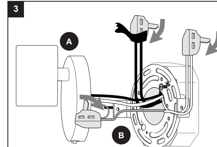
Connect wiring using preassembled lever wire connectors: WHITE to WHITE, BLACK to BLACK, BARE/GREEN to BARE.
