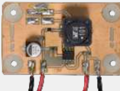
Figure 2. The small PCB for the LED driver. All components are SMD types.
