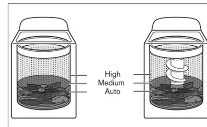
As the washer dampens and moves the load, the level of the items will settle in the basket.
