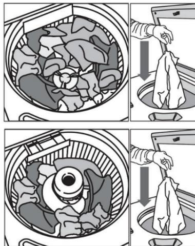
For best performance, it is recommended to load items by dropping them in loose heaps evenly around the washplate and agitator. Do not lay items length-wise around the washplate or agitator.
