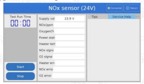
1)After connecting the oxynitride sensor, click the "Start" button to start the test. Nitrogen and oxygen sensors will be heated first. After about one minute, they will be heated to a certain temperature and stop heating. The oxygen concentration and nitrogen oxide concentration around the sensor will be
