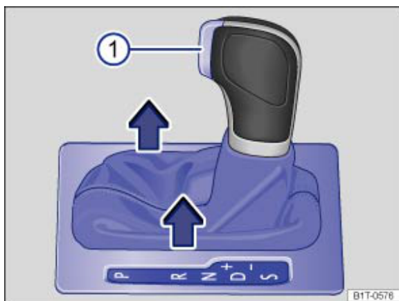
Fig. 220 Removing the cover of the gearshift gate
