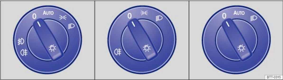
Fig. 87 Next to the steering wheel: examples of the various light switches
