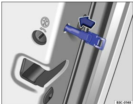
Fig. 215 Manually locking the vehicle with the spare key
