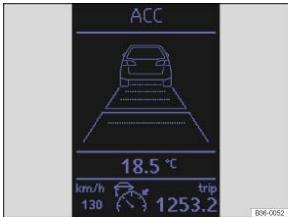
Fig. 167 Instrument cluster display: ACC switched off temporarily; vehicle detected ahead
