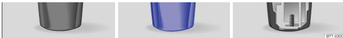
Fig. 24 Opening the battery cover on the vehicle key
