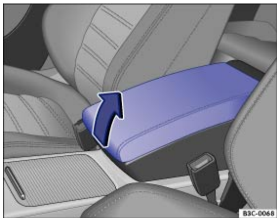
Fig. 120 Stowage compartment in the front centre armrest
