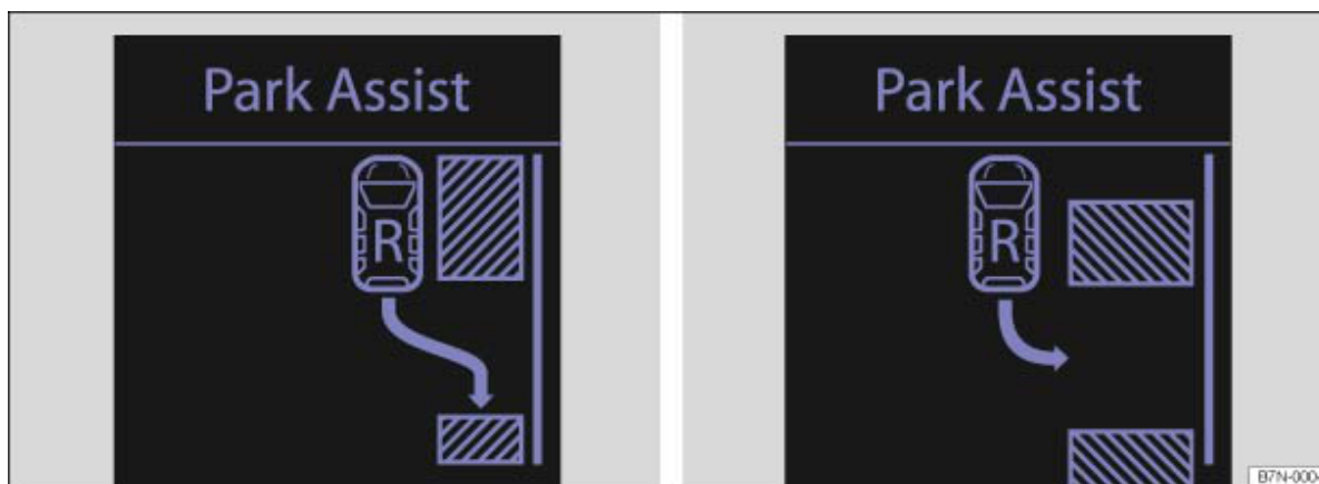
Fig. 159 Parking space detected: select the reverse gear for parking (perpendicular or parallel parking)
