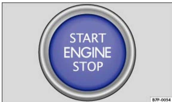
Fig. 137 In the lower part of the centre console: starter button for the Keyless Access locking and starting system
