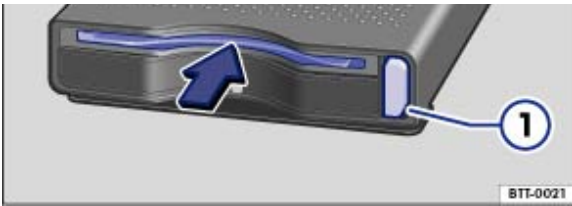
Fig. 135 In the stowage compartment on front passenger side: toll card reader
