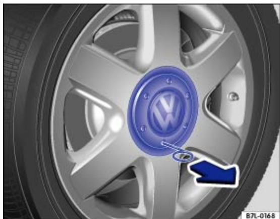
Fig. 224 Removing the centre covers by pulling
