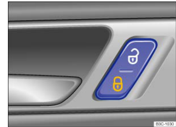
Fig. 27 In the driver door: central locking button
