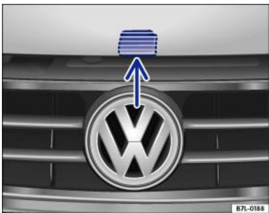
Fig. 193 Release lever for opening the bonnet above the radiator grille
