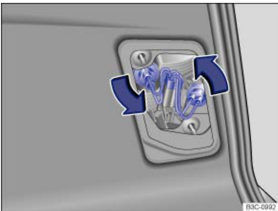
Fig. 247 In the boot lid: removing bulbs
