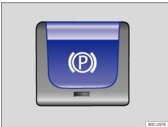
Fig. 146 In lower part of centre console: button for the electronic parking brake
