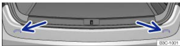
Fig. 106 In the luggage compartment: fastening rings
