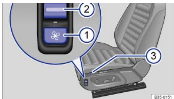
Fig. 54 On front seat: switch for seat ventilation
