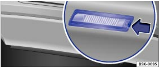
Fig. 250 In the rear bumper: number plate light
