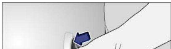
Fig. 33 In the driver door: release button for the boot lid
