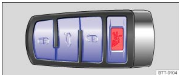
Fig. 20 Vehicle key with alarm button
