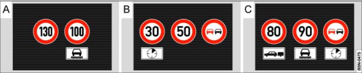
Fig. 177 In the instrument cluster display: examples of recognised speed limits or overtaking restrictions with accompanying additional signs
