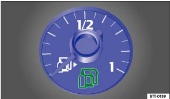
Fig. 187 In the instrument cluster: natural gas fuel gauge
