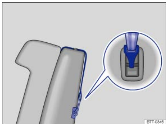
Fig. 79 Example of a fastened top tether
