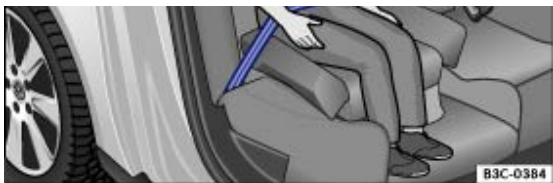
Fig. 83 Integrated child seat: seat belt routing
