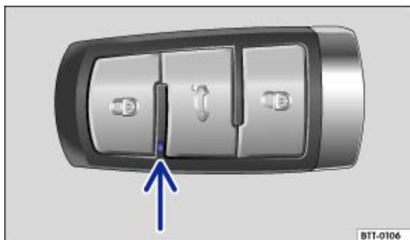
Fig. 22 Indicator lamp in the vehicle key
