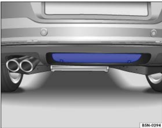
Fig. 114 Rear bumper: removing the cover
