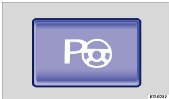
Fig. 158 In the centre console: button for switching on the Park Assist system manually
