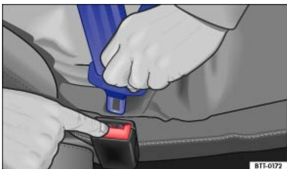
Fig. 66 Removing the latch plate from the buckle
