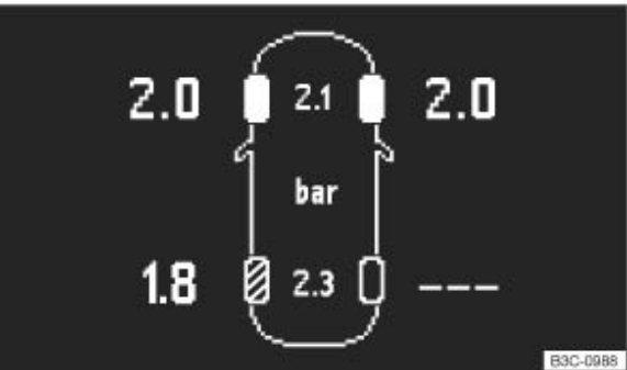
Fig. 180 Display in instrument cluster: current tyre pressures
