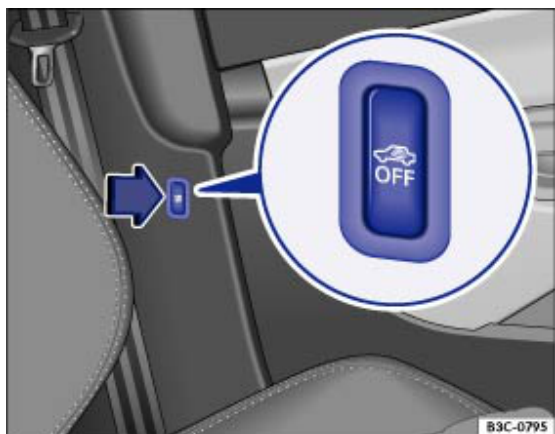
Fig. 30 Next to the driver seat: button for switching off the interior monitoring system and anti-tow alarm
