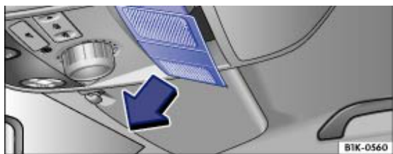
Fig. 218 In the roof: removing the cover
