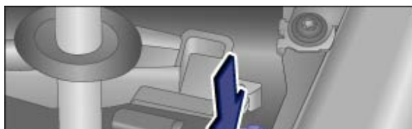
Fig. 220 Removing the cover of the gearshift gate
