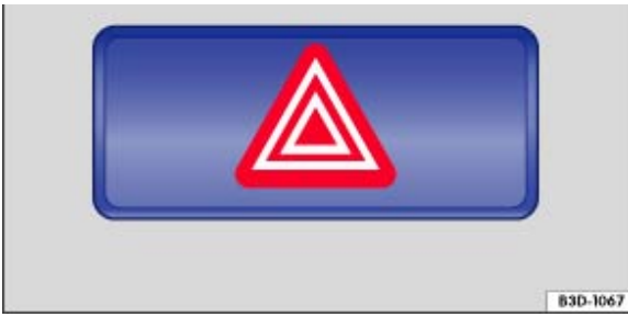
Fig. 211 In the upper section of the centre console: switch for the hazard warning lights
