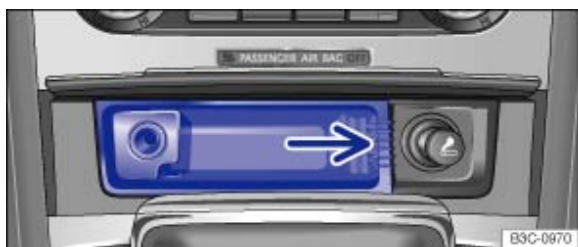
Fig. 129 In the front centre console: removing the ashtray
