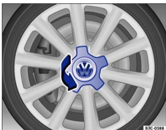
Fig. 225 Removing the centre covers by turning
