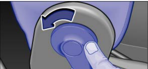
Fig. 56 Folding the front passenger seat backrest forwards
