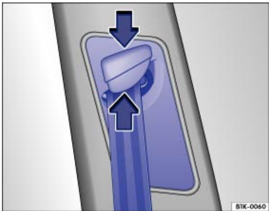
Fig. 69 Next to the front seats: belt height adjuster
