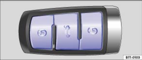
Fig. 25 Buttons in the vehicle key
