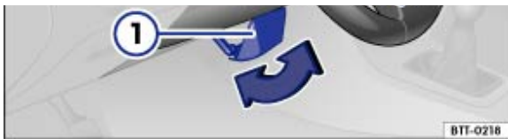
Fig. 49 Adjusting the steering wheel position mechanically
