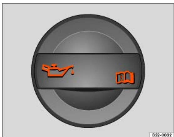
Fig. 195 In the engine compartment: engine oil filler cap
