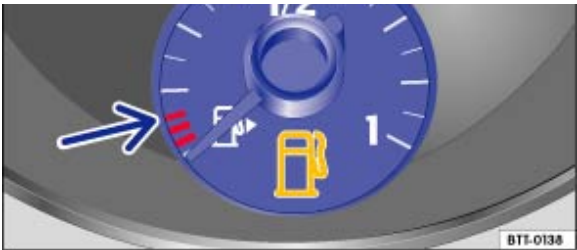
Fig. 186 In the instrument cluster: fuel gauge for petrol and diesel
