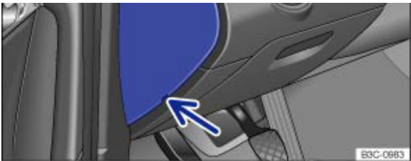
Fig. 238 Dash panel on the driver side: fuse box cover
