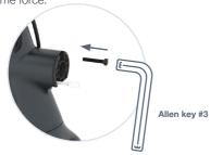
the Frame Bracket over the frame of the bicycle, with the flat side pointing towards the front of the bicycle. Make sure the brake cable is not caught between bracket and frame. Slide upwards so it does not touch the front fork.
