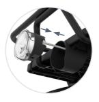
4.2 Gently pull the cable towards the front of the product, and stow away recess cable inside the light cover. Now slide in the front light (A) and fixate it with the set-screw, using anti-theft Torx #T10. (B).
