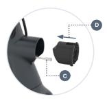
1.5 Screw the M5\*25 bolt with Allen key #3 tinto the frame. Tighten the bolt untill the adapter is fixated. this can take some force.
