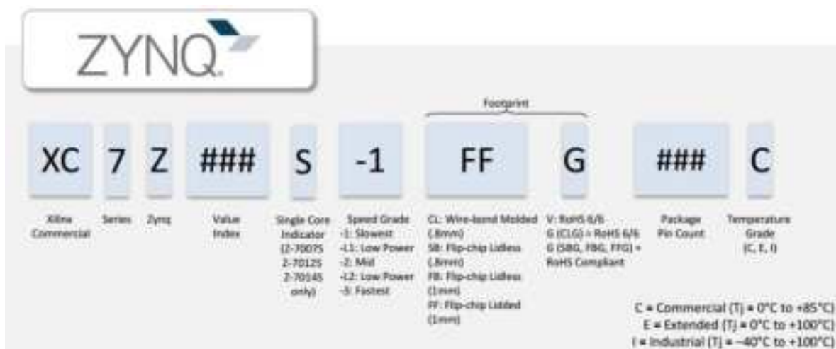
Figure 2-2: The Specific Chip Model Definition of ZYNQ7000 Series
