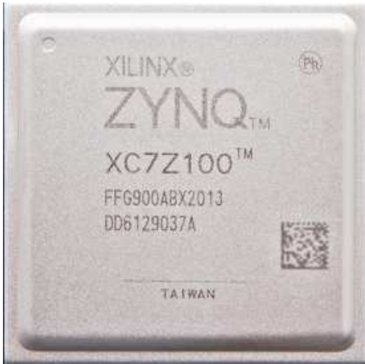
Figure 2-3: The XC7Z100 chip used on the Core Board
