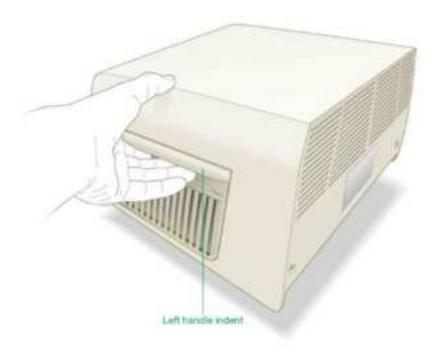
6. With its lid lever pointing toward the front, insert the reaction module into the reaction module bay, leaving about 2 cm of space in front of the thermal cycler.
