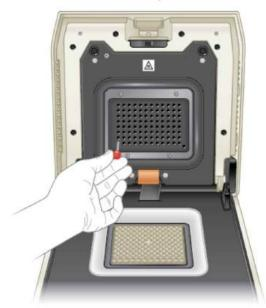
Note: You must reinsert the shipping screw should you need to return the reaction module for any reason. Save the screw in a safe and accessible place.
