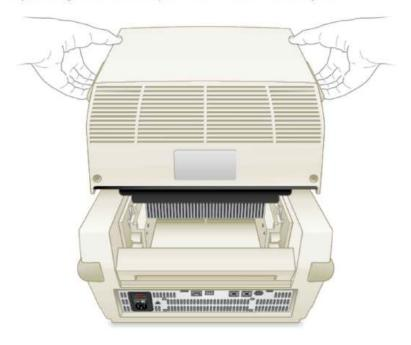
7. Pull the locking bar up to lock the reaction module in place.
