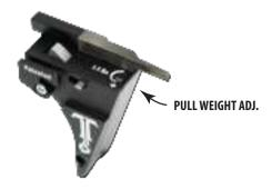
**IMPORTANT:** Your TriggerTech ACE Trigger System allows you to adjust your trigger pull weight. The set screw is located ontop of the Sear Module and is set to near the middle of the advertised pull weight range. To adjust pull weight, insert the supplied 5/64" Allen wrench. To increase pull weight, turn the set screw clockwise. Do not adjust your Sear Module more than 8 full rotations from the lowest pull weight.
