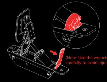
Insert the wrench into the back of the brake cylinder, then pull downward to loosen the cylinder.
