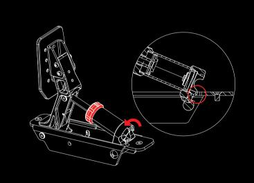
Flip the wrench and insert it into the back of the cylinder, then push upward to push the cylinder back in place
