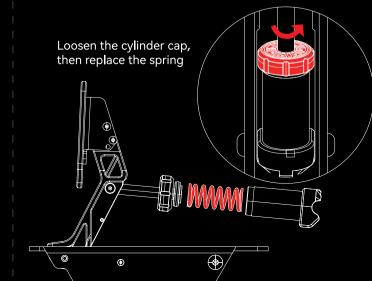
A brake washer can be added to improve brake feel (The washer is recommended for profile rig use only. Be cautious during the replacement process to avoid
