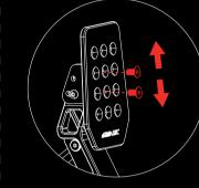
Loosen the two screws on the pedal front to adjust its height and position
