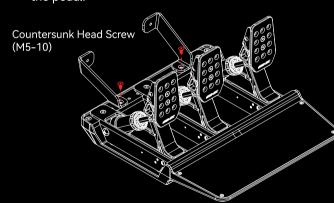
① Attach the wall plate to the left and right brackets, and tighten with two screws to complete the assembly.
