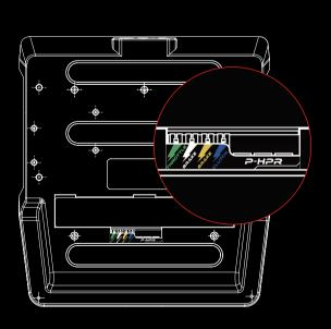
Invert the pedal to connect the cables, and plug the sockets into their corresponding colors
