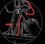
Use the included screwdriver to loosen the pin
