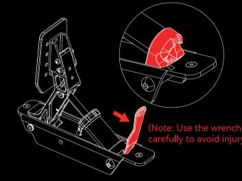
Insert the wrench into the back of the brake cylinder, then pull downward to loosen the cylinder.
