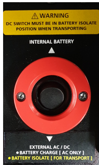
Figure 3.1 Battery select switch
