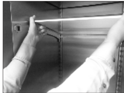
FIG. 3. Hook the shelves into the shelf standards.
