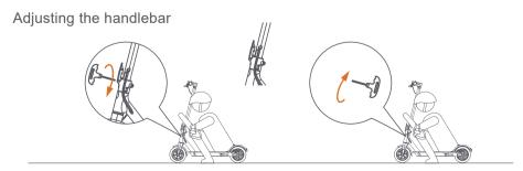
If the handlebar and its stem sway during riding, use the hexagon wrench to tighten the screws on the folding mechanism.
