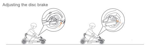
If the brake is too tight, use the hexagon wrench to loosen the screws on the caliper, and slightly send back the brake cable to shorten the exposed length, then tighten the screws. If the brake is too loose, loosen the screws, and slightly pull out the brake cable to lengthen the exposed length, then tighten the screws.
