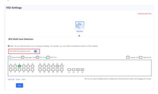
Click a port on which BFD is not enabled. Click Save to enable BFD on the port.
