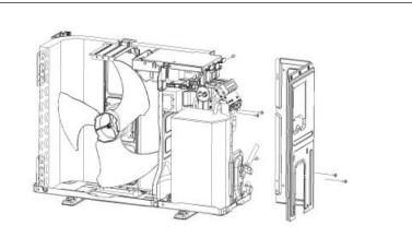
B Unfix the screws on the left plate, base plate, and condenser plate. You can then take the left plate out.
