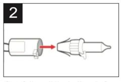
Carefully pull the bulb out of the socket.
