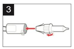
Insert a new bulb and lock the latch.
