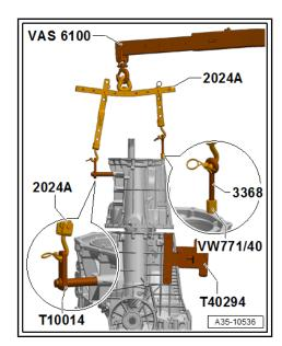
Lower the transmission intermediate housing into the transmission housing slowly and carefully.
