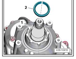
Install the shaft seal all the way around evenly using Seal Installer - Output Shaft - T40238- . Do not bend the seal.
