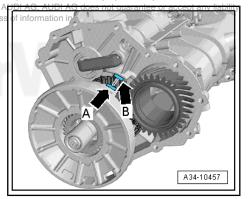
Place the center differential -2- on the transmission.
