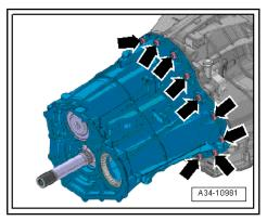
Engage the transmission intermediate housing -1- with the wheel set on the Shop Crane - VAS6100- as shown in the illustration.
