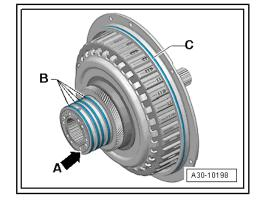
Remove the locking ring -arrow- with locking ring pliers.
