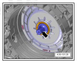
Slide the clutch module onto the input shaft -arrow- carefully without tilting it.
