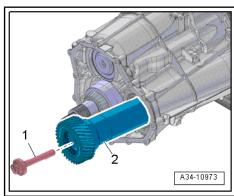
Remove the spur gear -1- and needle bearing -2- from the output shaft -3-.
