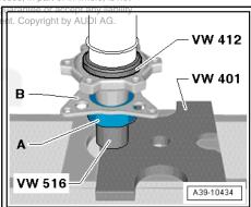
Install the circlip -1- in the flange shaft groove.
