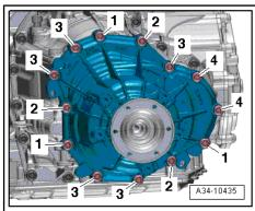
If the gear carrier -1- remains in the center differential housing, proceed as follows:
