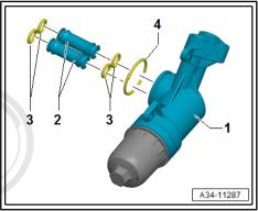
Carefully pull the ATF filter to the rear and off the Mechatronic in direction of -arrow-.
