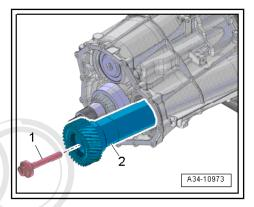
Insert the side shaft -B- all the way onto the pinion and into the transmission cover.
