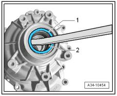
Remove the flange shaft ball bearing and spacer sleeve if necessary.
