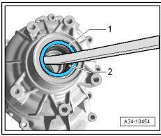
Remove the transmission output shaft ball bearing with splines, if necessary.
