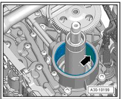
Coat the O-ring -C- and hub -B- on the dual clutch with ATF.
