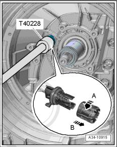
Remove the oil guide for the input shaft -arrow-.
