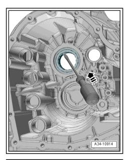
Position the new shaft seals for installation.
