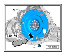
Turn the Puller - Clutch Module - T40176- upward.
