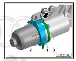
Remove the ATF filter -2- in direction of -arrow- and remove from below.
