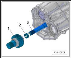
Insert the side shaft -2- with the bolt -1- into the transmission intermediate housing.
