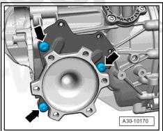
Remove the left flange shaft -2- from the transmission in direction of -arrow A-.
