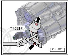
Mount the oil guide for the input shaft -arrow-.
