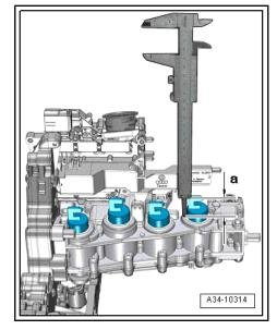
Align the gear selector yokes -arrows- so that they engage into the eyes in the shift fork when being installed.
