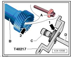
permitted unless authorised by AUDI AG. AUDI AG does not guarantee or accept any I Tighten the Counterhold in Side Shaftatiol. 402:12000 in the trans, AUDI A mission intermediate housing -arrows-.
