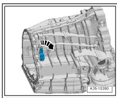
Make sure the alignment sleeves -1 and 2- are installed inside the transmission housing.
