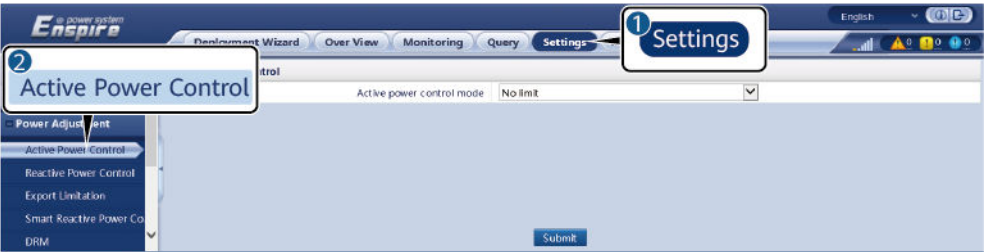
Figure 6-51 Active power control
