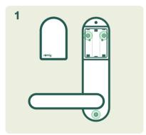
Prepare your inside unit for the installation. On most models, there are **two (large) screws** in the battery holder and **one** on the underside.
