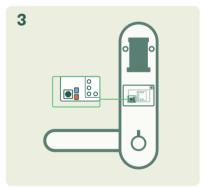
The module enters pairing mode automatically for **four minutes**, indicated by **orange (zigbee)** and **blue (bluetooth)** flashing from the module.
