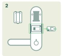
**Carefully** install the module in its slot on the inside unit. The batteries should be removed during installation.
