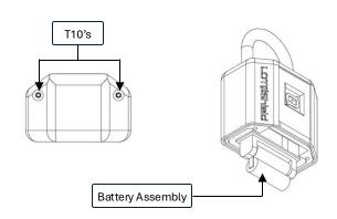
Note: Under ordinary use, the batteries are estimated to have a lifespan of approximately one year. You may order newbattery assemblies at: www.lot0shield.com/order/battery
