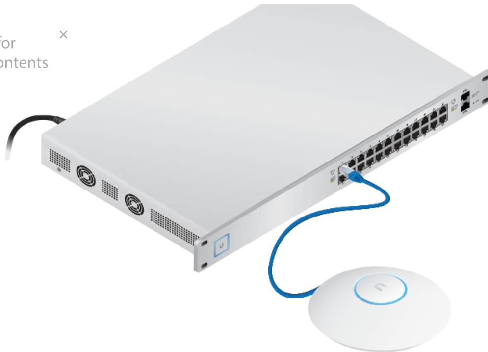
UniFi Switch with PoE Power Connection Diagram
