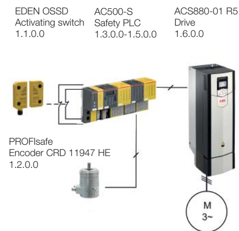
Figure 2: Connection example of the safely-limited speed function with an ACS880-01 and an AC500-S safety PLC.
