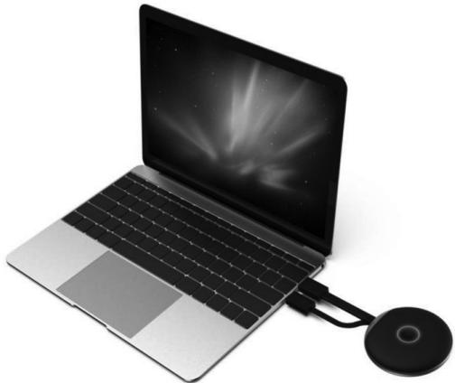
The edge of the control button lights up red immediately after the USB connector has been inserted. The device initialises and establishes a wireless connection to the base station. If the HDMI connection is connected correctly, the colour changes to purple or blue (flashing).
