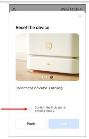
3) Once it is confirmed that the **Wi-Fi indicator**  $\mathfrak{I}$  (15) is flashing slowly, touch "**Next**" and "**Add**" to finish. The device is now added into the APP.
